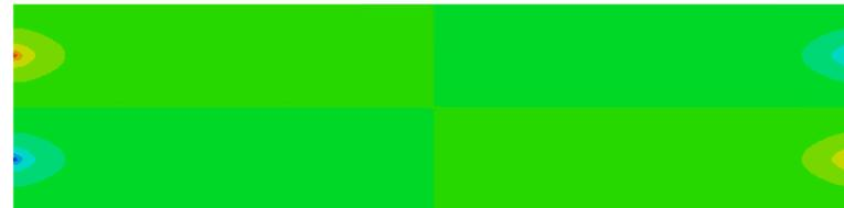
$\sigma_{xz}$  in an angle-ply laminate ( $\pm 45^\circ$ )s under uniaxial extension [1]
