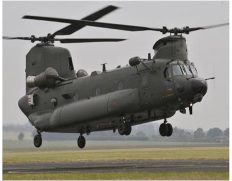
Length: 8.6 m Chord: 0.72 m. D-spar: 60 graphite/epoxy plies Ply thickness: 125 microns
